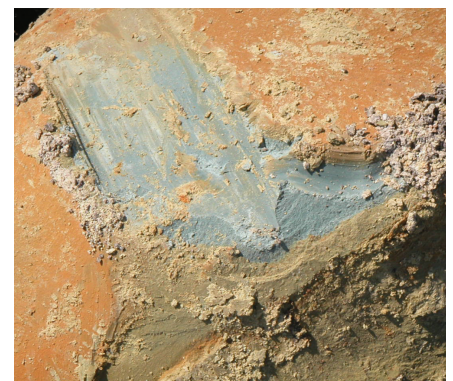
Figure 1: Turkish bentonite, illustrating oxidised yellow rind around remnant blue bentonite core. The yellow bentonite has improved drilling product performance.
