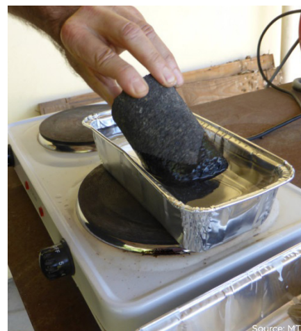
Figure 3. Coating a friable chromitite core sample with molten paraffin wax.
