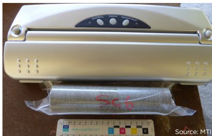
Figure 4. Vacuum-packing a pyroxenite core sample.
