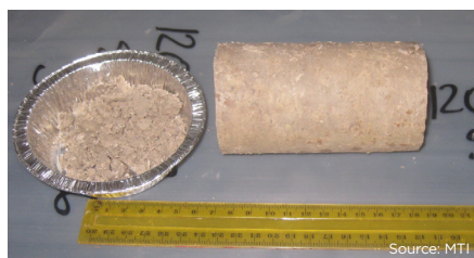
Figure 6. Bentonite core trimmed for calliper method and core 'shavings' for moisture analysis.
